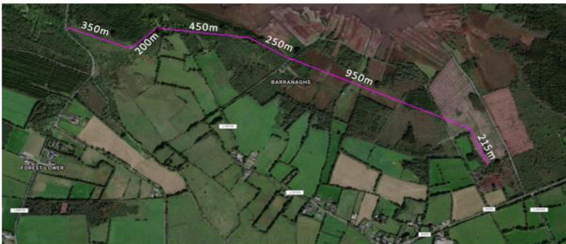
Figure 3 Wind Farm Collector Cable and access track
