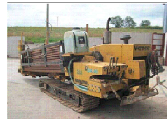
DIRECTIONAL DRILLING RIG
